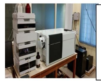
Liquid Chromatography-High Resolution Mass Spectrometry (LC-HRMS)
